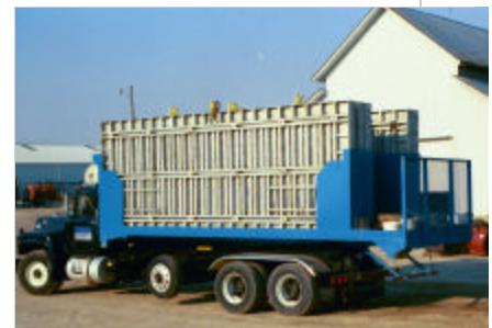
TJ's hauler is also equipped to hold other jobsite supplies along with their forms.
