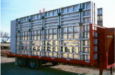
Pair of 4' x 18', male panel on top, female on bottom, with storage for POWER Ties bolted together for quicker setting & stripping.
