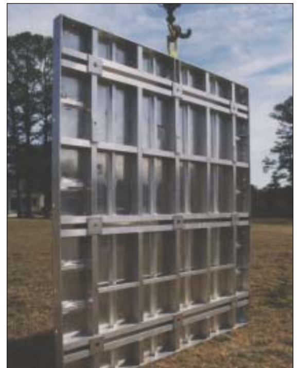
BIG PANELS make quick work of tall wall projects minus the labor for ganging handset panels together.
